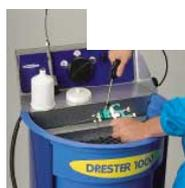
The rinse gun is designed specifically for effective high-pressure cleaning of spray-gun paint channels. It is as standard set to use fresh water, but can easily be set for recycled water.
