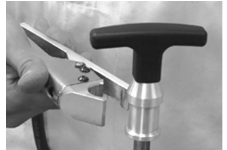
❸ Fit the clamp on the tool
