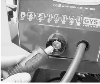
❶ Connect to the generator
