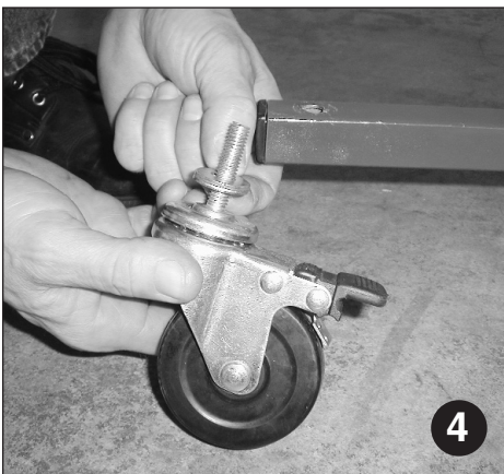
4 Tube bending during manufacturing can not be exact every time; 3/8" washers may be needed to shim wheel.
