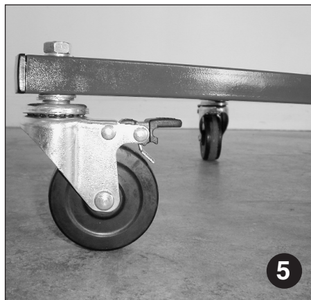
5 Photo shows installed shims (the 3/8" washers).
