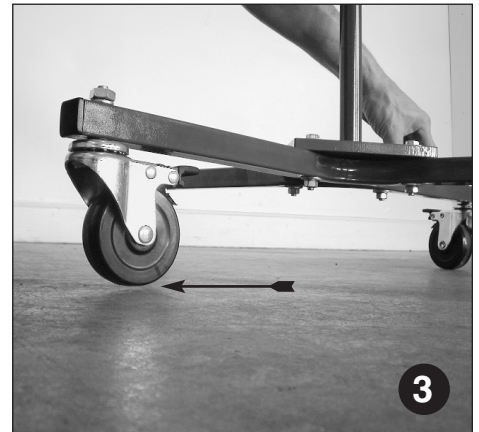
3 Check to see if all wheels are making contact to floor. Photo shows wheel slightly off of floor.
