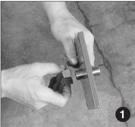
1 Screw connector into base plate 5/8" through other side, then tighten large nut firmly. Install bottom post tube. Note: use Loctite on all threads.
