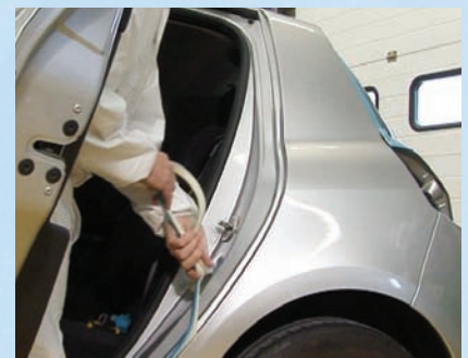
Once painted and baked, remove 3M Soft Edge Foam Masking Tape PLUS and remaining masking products.
