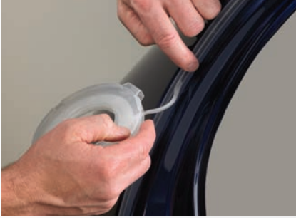
Masking jambs/apertures for highest quality repairs.
