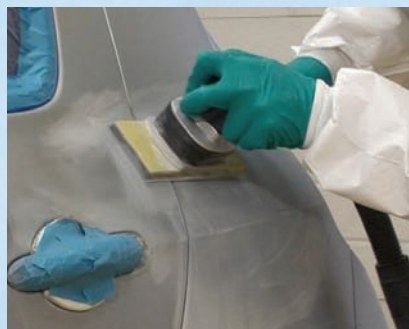
Sand the primer and blow down and degrease in the normal way.
