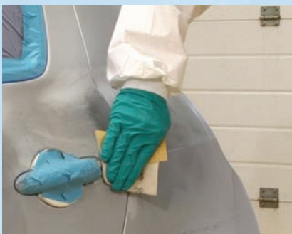
With 3M Soft Edge Foam Masking Tape PLUS and remaining masking still in place
