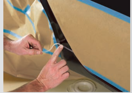
Feathering stone chip coatings.
