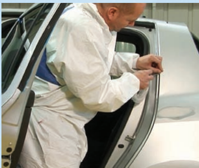
Apply to the edge of the door jamb where the primer line should stop.
