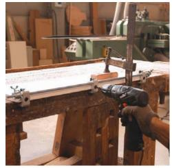
Template for wood pin joint (8 mm). High precision system with no need of side regulation required.
