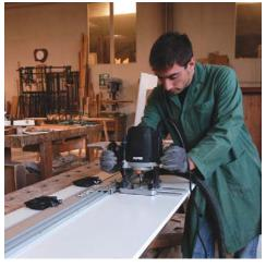
The 9.D310/C guide rail lets a safe and accurate straight power tools guidance. It is provided with two rubber suction pads and two fastening clamps to hold it
