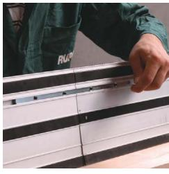
Provided with antislip strips to hold it firmly and to prevent scratches on the
