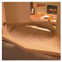
The template can be firmly fasten with the two rubber suction pads with to avoid holes on the surface.
