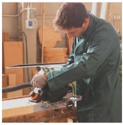
The tilting fence lets the planning work on orthogonal and angle edges.
