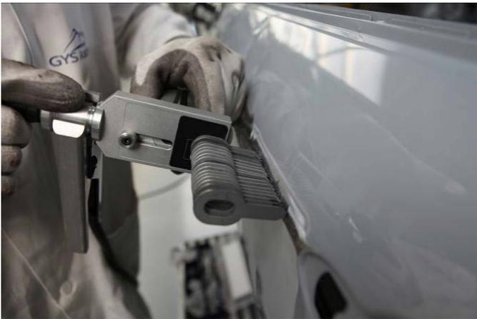
The RINGMATIC can be used with all dent pulling machines with automatic detection in the market using a simple "click" connection.
