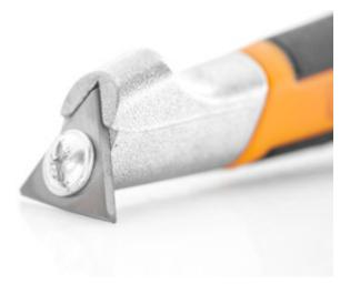
The three-edged plastic cutter is used to the repair process with PLASTOFUSED. It is designed for roughenung the plastic parts before welding. The advantage here is to get a better fusion of the thermoplasts.
