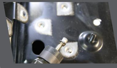
Weld extractor studs for the removal of punch rivets quickly and safely (separate tool required)
