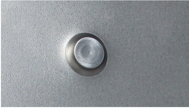
RESULT OF THE INSTALLATION OF SELF-PIERCING RIVET
