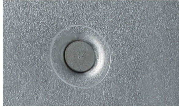
RESULT OF THE INSTALLATION OF SELF-PIERCING RIVET
