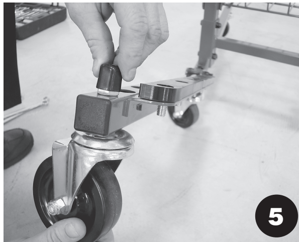
Install protective rubber cap. Adhesive can be used to better keep rubber cap in place.
