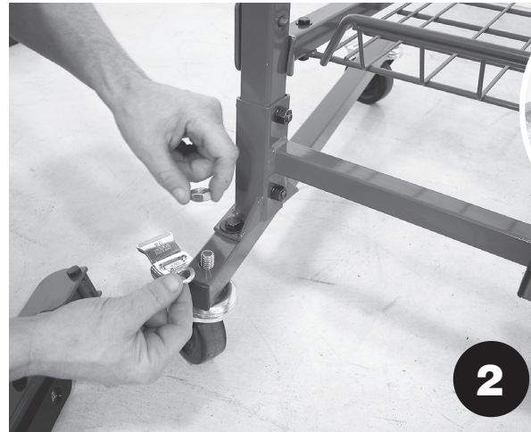
Remove rear wheel caster nut from cart and discard lock washer.
