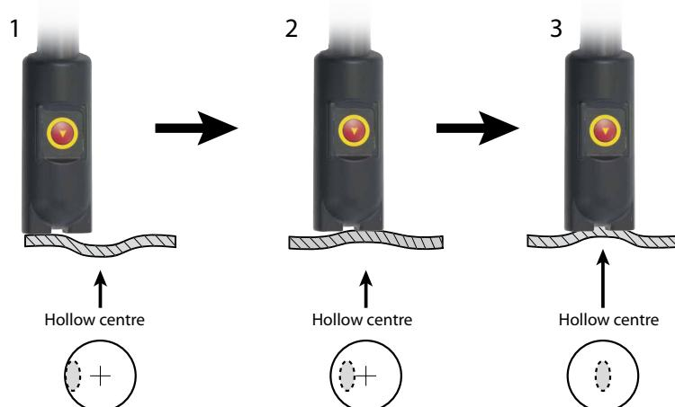
In certain cases the dent depth might increase whilst being heated (the sheet metal can go down as a result of the heat). If this is the case, increase the heat on the perimeter of the dent and continue to heat until it starts to decrease. For deep dents, heat in a circular motion around the dent, towards the centre.
