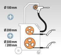
**2 torches, 2 integrated wire feeders + 1 Spool Gun** - The M3 GYS AUTO is a multifonction and flexible machine designed to weld 3 different types of wire at the same time. It saves time since it does not require to disassemble the torch and change the wire reel for another job.
