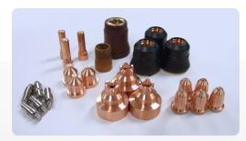
During cutting, consumables are subject to extreme heat, around 2000°C. They will then deteriote progressively after each use, affecting the pressure and cutting quality. It will then be necessary to replace sooner or later some consumables to get back to an optimum cutting quality.
