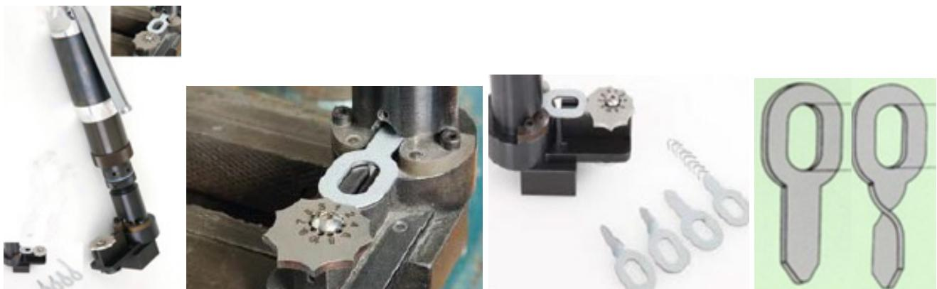
The pneumatic bit sharpener allows cutting the tip of pulling bits (pulling rings) in order to avoid complicated and tedious grinding of the bits one by one. Each bit can be sharpened up to 10 times.
