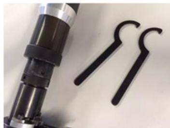
The 2 keys provided allow adjusting the height of the punch. In order to increase the height of the punch, in case there is a ball at the extremity of the bit, the upper part of the tool should be unscrewed. Adjust the height of the punch as desired. Then block the position of the upper part using the lower ring, with the 2 provided keys.
