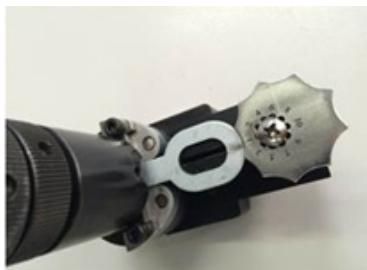
The back part of the bit should touch the plate with numbers, like shown on the photograph left. The numbers on the plate correspond to the cut length of the bit. The first time the bit is sharpened, the plate should be placed on position 1. For the following times, increase the number on the plate in order to cut the bit further up. The higher the number on the plate, the shorter the bit will be.
