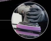
Combined circular and oscillating motion eliminates swirl marks and other defects
